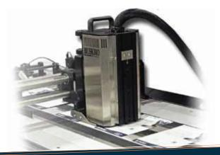
These printheads are equipped with Buskro's TrueFlow ink management system, which combines a simplified ink path and proven ink delivery that allows ink to flow effortlessly and efficiently to the print modules to produce quick start-ups, maintain print sustainability, and ensure rapid jet recovery.
